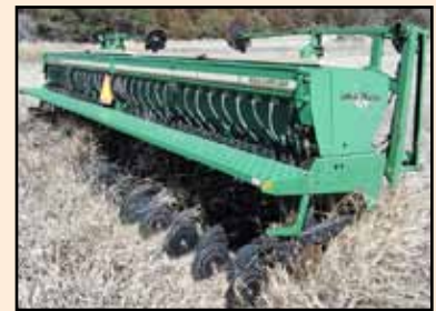
Great Plains Solid Stand 2000 3 pt. Drill 20 ft. 7 1/2 in. sp, markers, grass seeder
